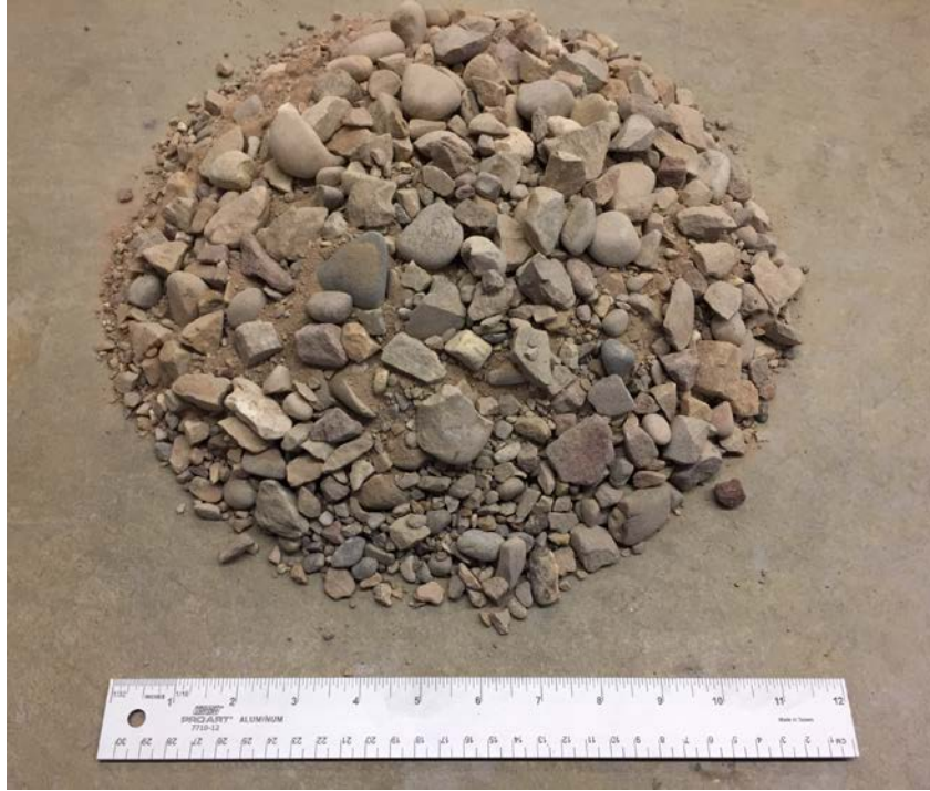
Figure 3-3: Wells Draw Road aggregate base material.
