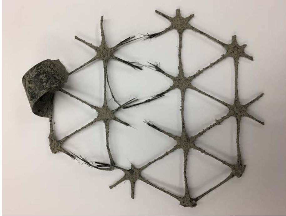
Figure 4-2: Geogrid rib failure.
